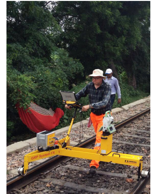
Track survey in India with Amberg IMS-system: production speed of 4 kmh.
