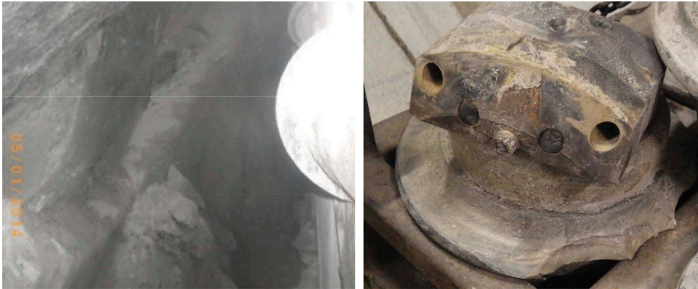
Figure 1. Left: Block rock mass. Right: damaged disc cutter, after operation in such conditions.
